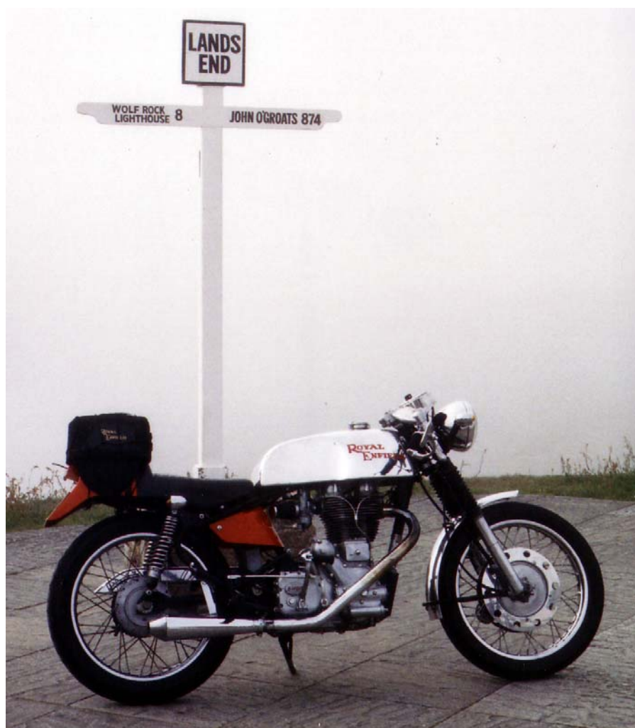
The Bullet has an alloy barrel and 9:1 high-compression piston Only 1/2 pint of oil was lost thanks to Hitchcock's 'breather kit' recycling oil back into the oil tank.
